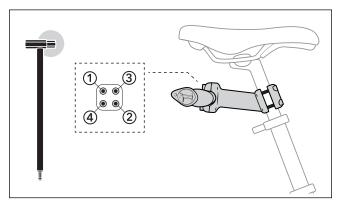
Tighten bolts in cross pattern to a torque of 9-10 Nm.
